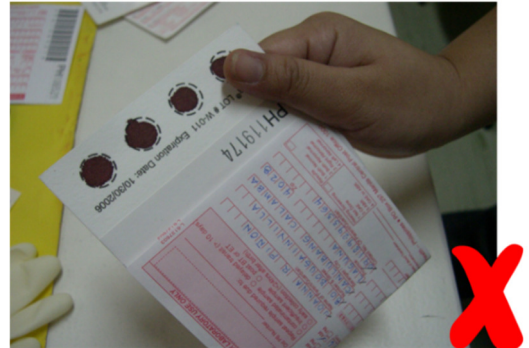
Figure 18. Improper handling of filter card.
