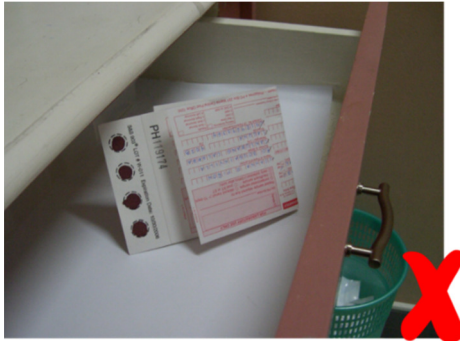
Figure 17. Improper storage of filter card.
